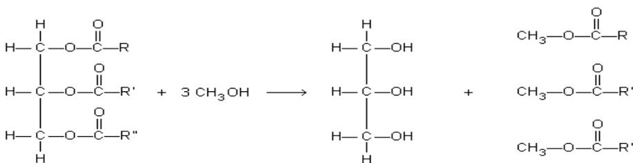
The biodiesel is made up of a mixture of the esters of the fatty acids that were present in the vegetable oil used.
