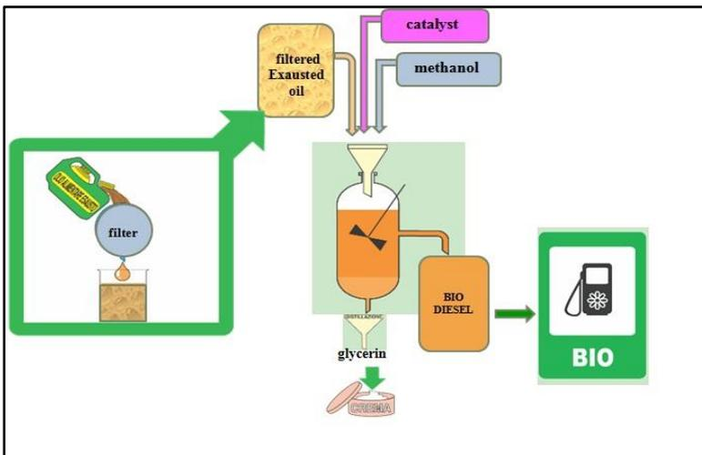
At first the oil is filtered to remove food residue, the filtered oil is put into the reactor with methanol and a base (usually NaOH *sodium hydroxide*). The reaction can be carried out at low temperature. From the reaction are obtained biodiesel and glycerin. The glycerin is not only a byproduct, but itself represents a useful product in the pharmaceutical and cosmetic industry.
